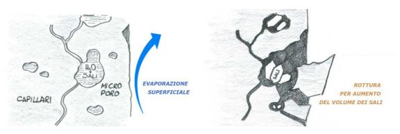
Fig. 1: Deposit of salts in the pores
