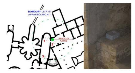
Fig. 7: Installation of the first device
