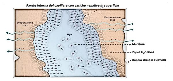
Fig. 2: Schematic representation of the "Helmholtz double layer"
