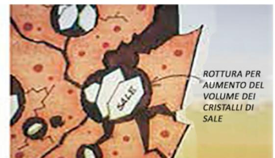
Fig. 6 - Deposit of salts in the pores.
