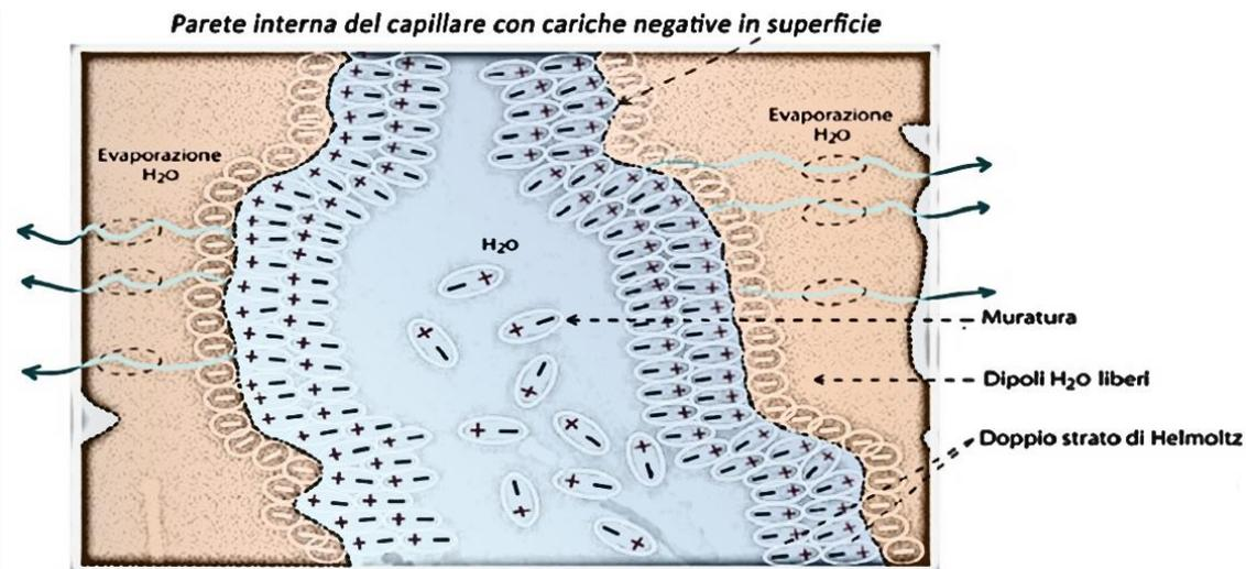
**Fig. 2:** Schematic representation of the "Helmholtz double layer"
