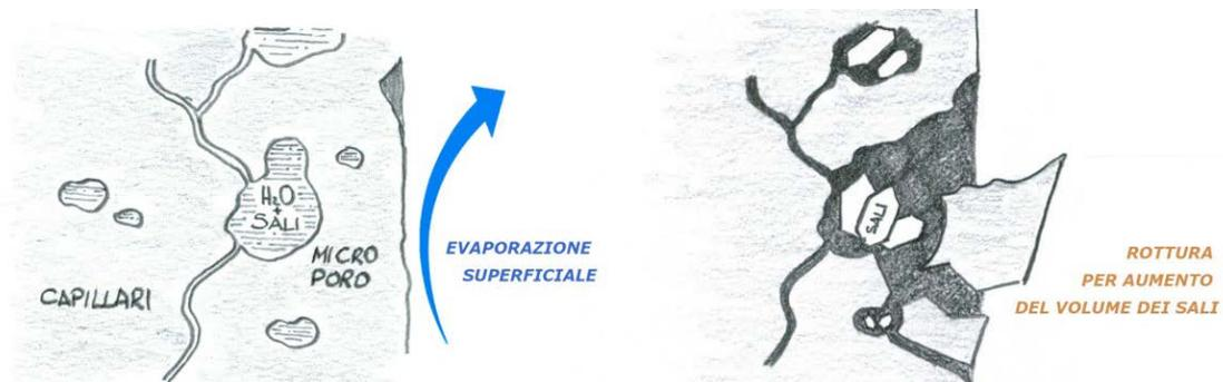
Fig. 1: Deposit of salts in the pores
